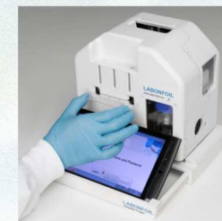
SmartCard lab-on-a-chip device for real-time PCR detection of food borne pathogens, marine algae analysis, climate change and Colorectal Cancer patients monitoring (LABONFOIL Project)
