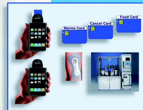
SmartCard lab-on-a-chip device for real-time PCR detection of food borne pathogens, marine algae analysis, climate change and Colorectal Cancer patients monitoring (LABONFOIL Project)
