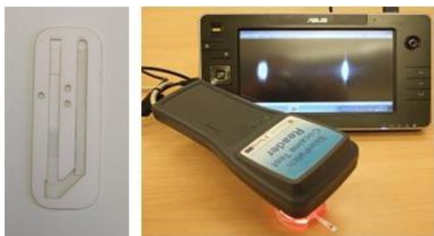
Fig. 5: Pictures of the developed labonapaper (left) and its reader (right). Pictures from Biosensia and PWR.
