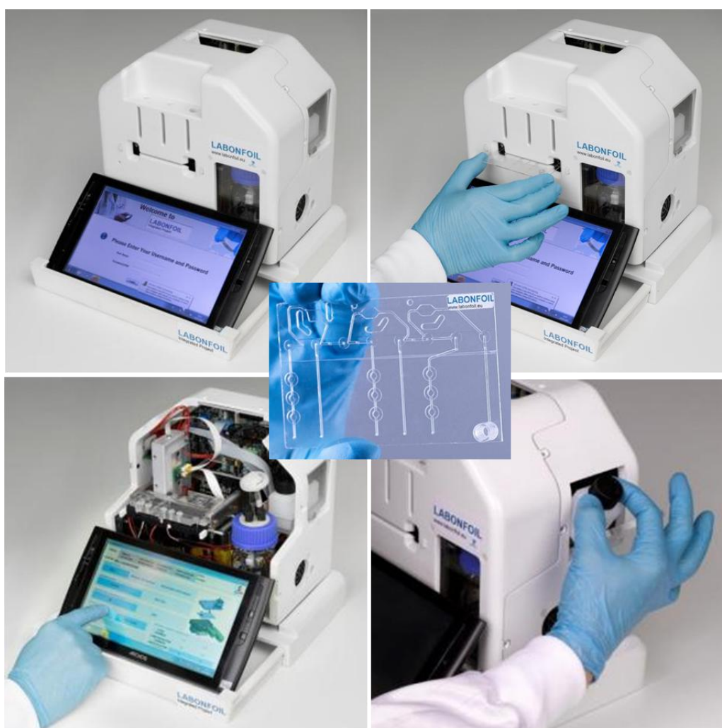
Figure 2. LabCardReader prototype pictures. Ikerlan-IK4 pictures. In the middle it can be seen the picture of the labcard.
